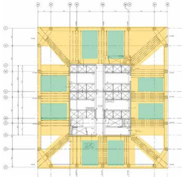
**Fig. 2: Plan of typical high-rise (tower) level (Note: Green designates area of future stair opening, additional slab reinforcing is required; yellow designates no future slab penetration is these areas, limited small sleeves may be allowed; and white designates area for small penetration, sleeves, and poke-throughs)**
