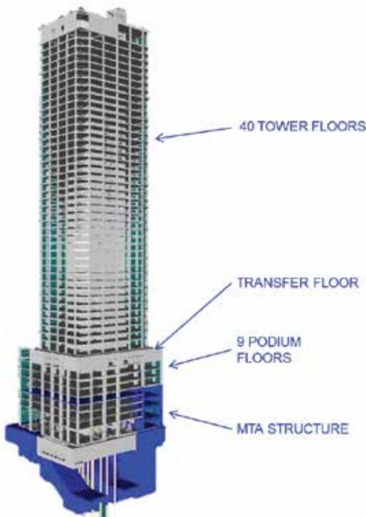
Fig. 5: Structural model of 55 Hudson Yards
