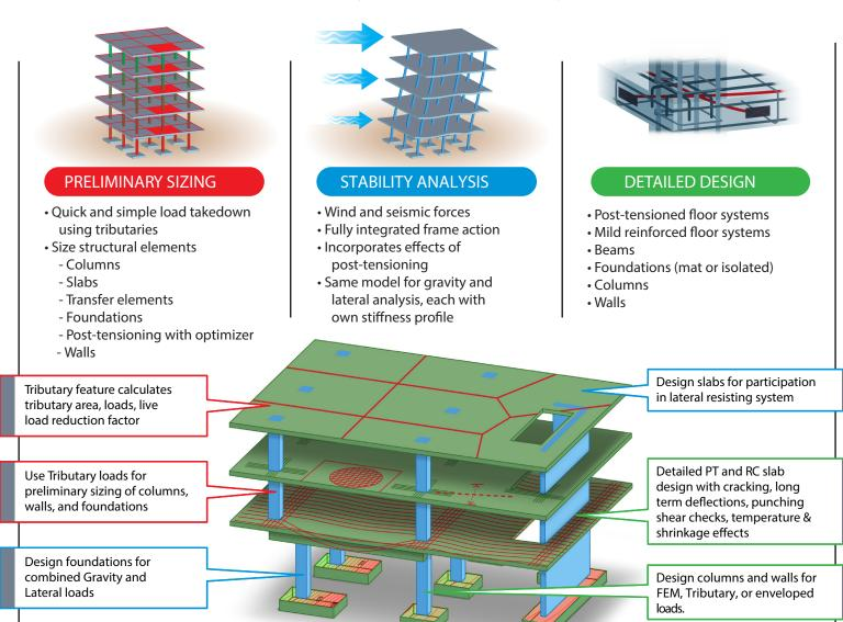
ADAPT-Builder is specifically designed for the rapid modeling of concrete structures and gives the option of adding prestressing or post-tensioning to any slab or beam member at any level. Directly import concrete building models from ETABS, Revit, or CAD, or use your Builder model to generate a new Revit Structure model.
